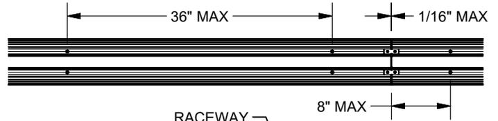
SELECT A STYLE OF EDGE TO BE USED IN THE RACEWAY BASE. USING A RUBBER Mallet OR BUTT OF RUBBER-HANDLED HAMMER, SNAP RACEWAY BASE EDGES INTO THE RACEWAY BASE.
